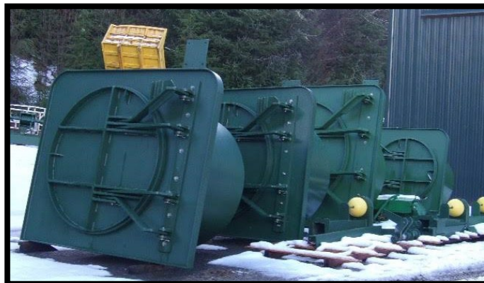
March 2023 – Tide gates fabricated and ready for delivery.
