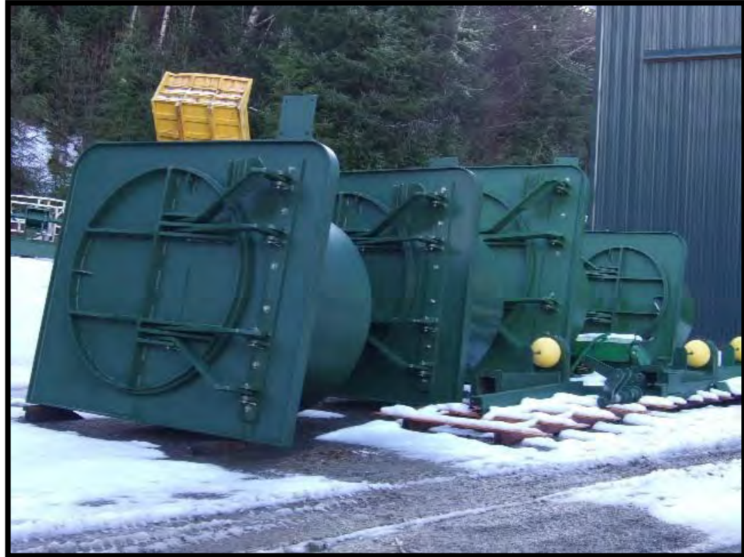
March 2023 – Tide gates constructed at Nehalem Marine and ready for delivery to the Glover Ranch.
